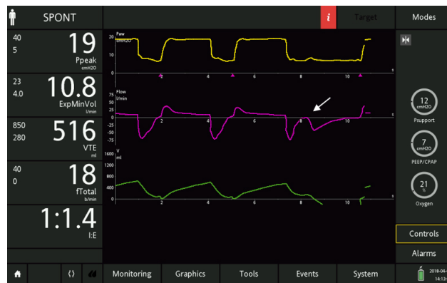
Figure 9: The same patient ventilated with inspiratory trigger sensitivity: 2 l/min, expiratory trigger sensitivity: 25%, ramp: 75 ms (top), immediately after changing the ETS to 10% (middle; red line), and after a few breaths with ETS at 10% (bottom). Note the prolonged inspiration with evident late cycling in the first breath after the settings have been changed (red arrow), and the effect on the triggering phase soon leading to ineffective efforts (white arrows).
