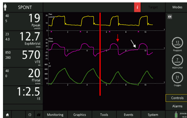
Figure 10: The same patient ventilated with inspiratory trigger sensitivity: 2 l/min, expiratory trigger sensitivity: 25%, ramp: 75 ms (top), and after changing the ETS to 45% (bottom; red line). Note the correction of delayed cycling to expiration (red arrow) and the shorter inspiratory delay (white arrow), thus confirming the asynchronies’ interdependence.
