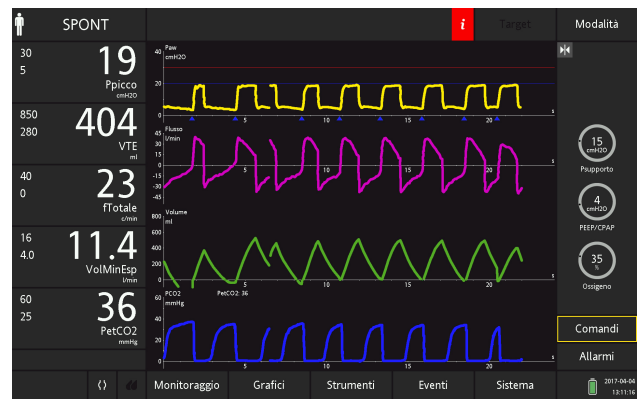
Figure 17: The same patient after activation of IntelliSync+. Note not only the resolution of late cycling and the elimination of ineffective efforts, but also the curves’ appearance, which changes slightly from one breath to another, as happens physiologically.
