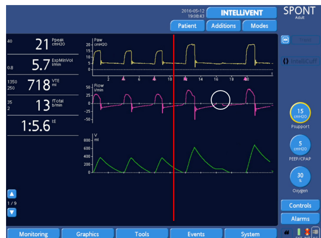
Figure 13: Next step representing an increase in the level of pressure support (from 10 cmH2O to 15 cmH2O; red line). Late cycling appears again despite the high ETS, followed by an ineffective effort (circle). At this point, reoptimization of settings would be necessary.
