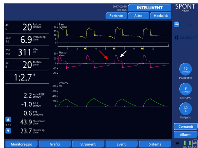
Figure 6: The same patient ventilated with inspiratory trigger: 2 l/min, expiratory trigger sensitivity: 25%, ramp: 75ms (top) and after switching to pressure trigger: -2 cmH 2 O, but keeping the other settings as they were (bottom). Note the increased inspiratory delay (red arrow) and, as a consequence, late cycling to expiration (white arrow).
